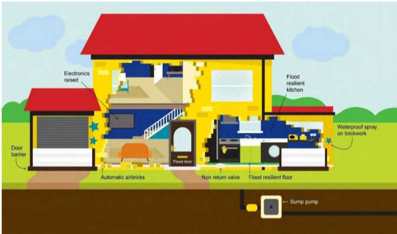
Figure 1-3 examples of Property Flood Resilience techniques
